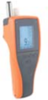
Figure 3 – Digital Electronic Dewpoint Meter
