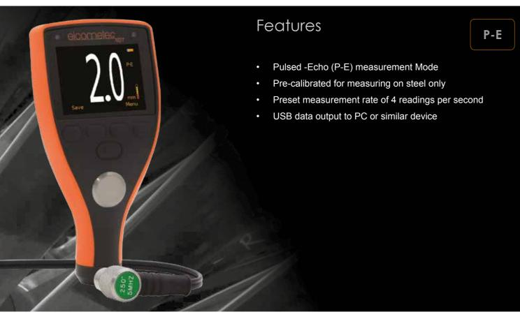
With automatic transducer recognition, which ensures correct probe identification even when the transducer is changed, a measurement rate of 4Hz (4 readings per second) and integral zero disc, ensuring maximum accuracy of ±1%, the MTG2 is ideal for taking basic thickness measurements.
