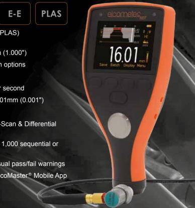
The PTG8 has Differential Mode; once a user defined nominal thickness value is set, the gauge displays the measured thickness together with the variation from the set nominal value thus indicating areas of the material which are thinner or thicker than expected.
