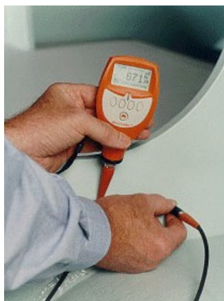
Figure 2 – Measurement of coating thickness
