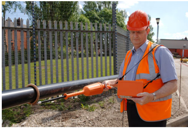
Figure 10 – Rolling spring probe in use on external pipe coating
