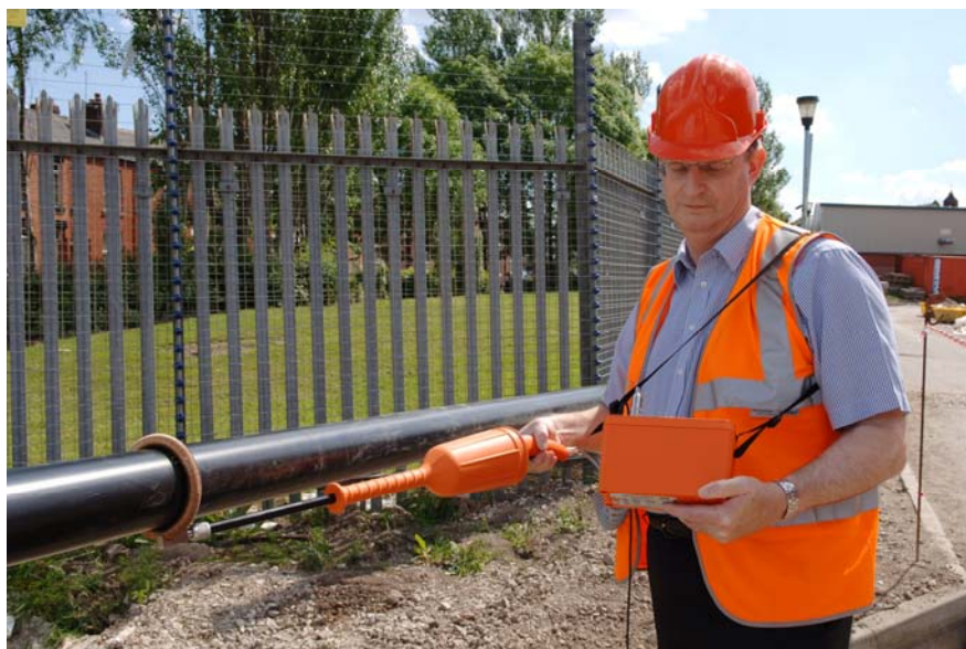
The Rolling Spring Electrode in Use on a 150 mm Diameter Pipe The High Voltage Handle is fitted with an Insulated Second Handle to Aid Handling
