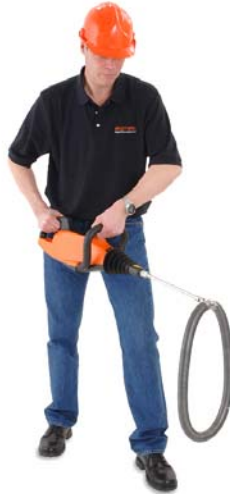
The Pulsed DC High Voltage Holiday Detector Showing a Rolling Spring Electrode Ready to Wrap Round a Pipe.
