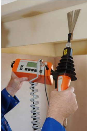
A Continuous DC High Voltage Porosity Detector Being Used with a Band Brush Probe on a Coated Beam
